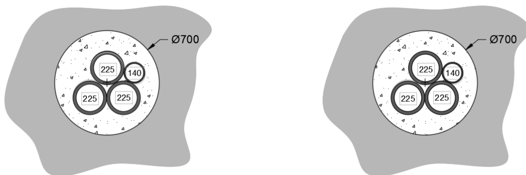
Figure 2 – Indicative HDD duct formations
